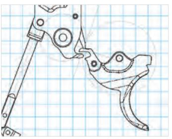
Patented Friction-Reducing Cam
